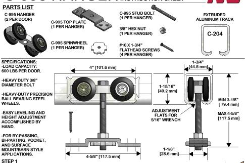
DETERMINE DOOR SIZE/HEADER HEIGHT BASED ON DIMENSIONS SHOWN IN DETAIL VIEWS AND CLEARANCE REQUIRED BELOW DOOR. NOTE: DUE TO STUD LENGTH, THE C-995 HANGER IS USUALLY INSTALLED FULLY ASSEMBLED ON THE DOOR. THE COMPLETE ASSEMBLY IS THEN "LOADED" ONTO THE TRACK FROM ONE END. FOR BI-PARTING APPLICATIONS IT IS RECOMMENDED THAT THE TRACK BE INSTALLED IN TWO PIECES. MOUNT ONE PIECE TO THE HEADER, LOAD BOTH DOORS INTO TRACK, AND THEN INSTALL SECOND LENGTH OF TRACK.
